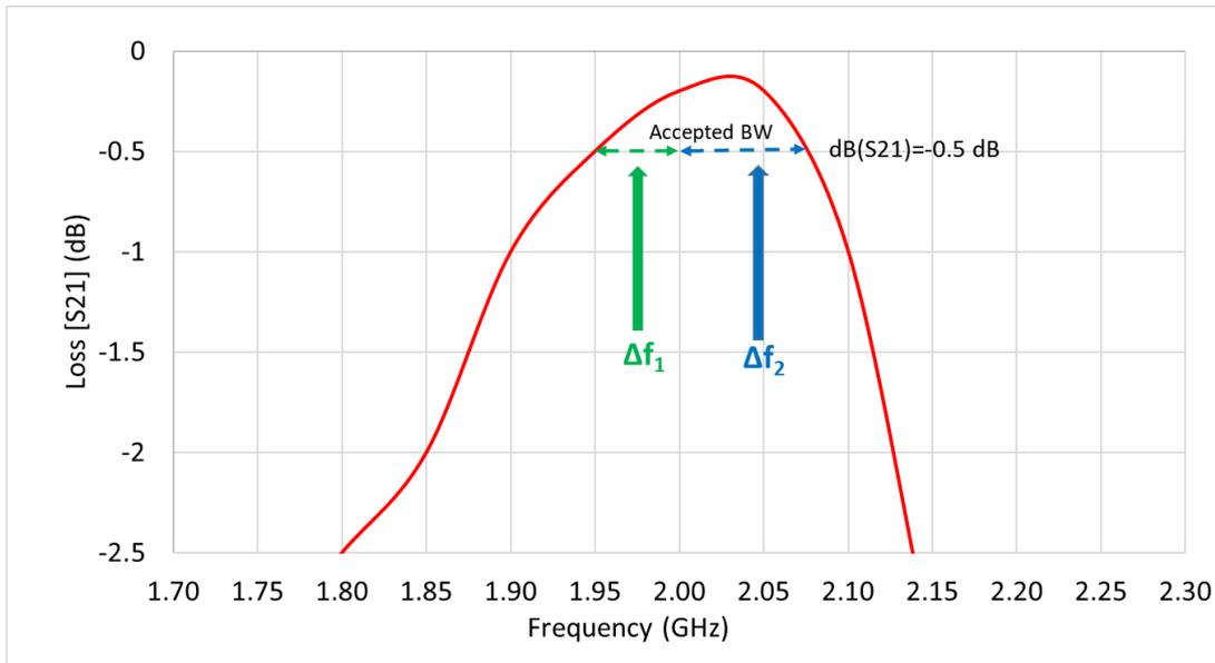
**Figure 2.** Insertion loss measurement.
