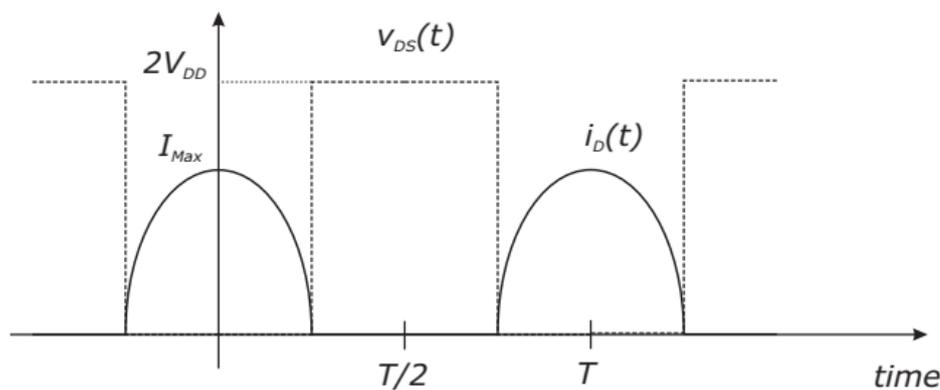
**Figure 1.** Ideal voltage and current waveforms for a Class-F amplifier [1].
