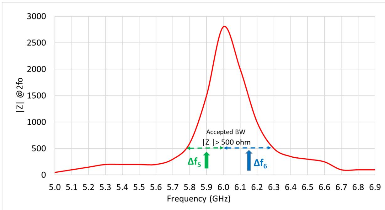
**Figure 4.** Impedance measurement at 3<sup>rd</sup> harmonic frequency 6 GHz.
